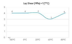
The graph below shows the results of thermal aging. The adhesive was aged at the indicated temperature, tested at 22 ° C (71.6 ° F) and cured for one week. Lap shear strength has been tested in accordance with ISO 4587 on shot blasted mild steel (GBMS).
